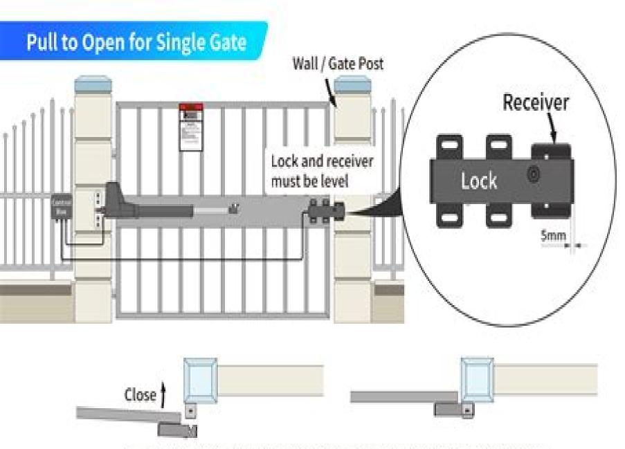
Lock and Receiver must fit close. Check it when the gate closes firmly.
