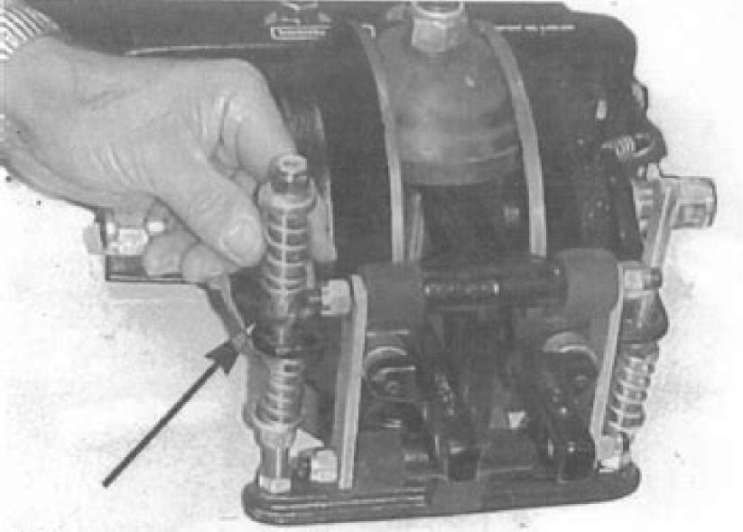
NOTE: Convex or rounded side of the washer goes down
