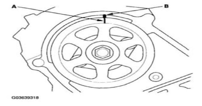
Fig. 40: Alining TDC Marks On Camshaft Pulley With Pointer (Rear)
