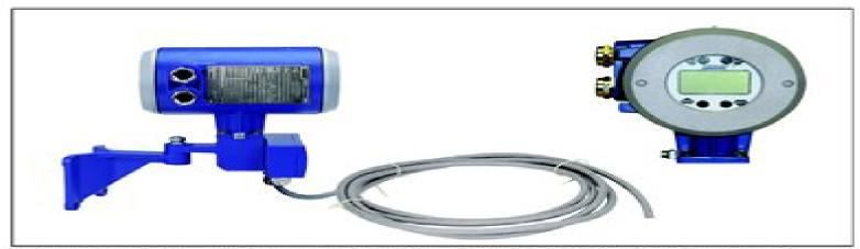
The Model CFT50 Digital Coriolis Mass Flow Transmitter combines with a Model CFS10 or CFS20 Mass Flowtube to form an I/A Series Mass Flow and Density Meter. This transmitter is a digital device as compared to the analog architecture of earlier transmitters. Use of digital signal processing (DSP) techniques improves flowmeter performance and minimizes the shortcomings experienced by existing transmitters. The CFT50 uses HART protocol for remote communications.
