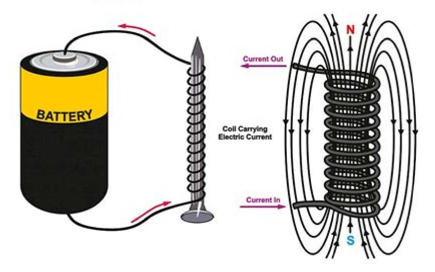
Electromagnet is a temporary magnet that produce a magnetic field when regular electric current passing into a coll.
